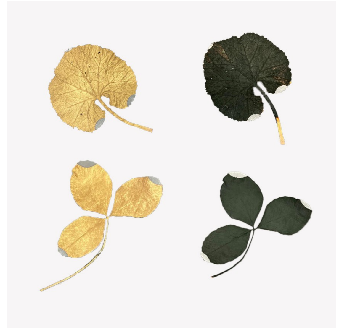
Bioinspired artificial muscle-sensor based on conducting polymers functionalized electrospun fiber networks on decellularised plant tissue (with Mihaela Bunea, Mihaela Beregoi)
